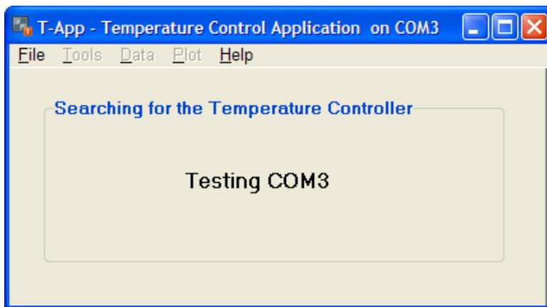
When a **Controller** is found, this startup window is replaced by the [Application Control Window](#).
