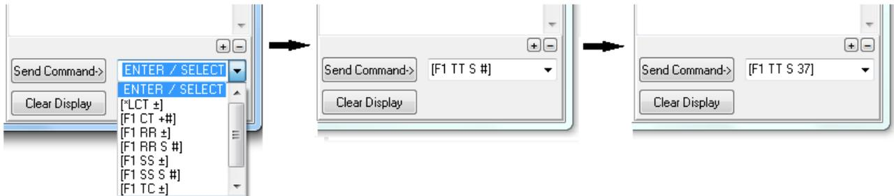
To send the command to the QNW Temperature Controller either hit the Enter key on the keyboard (while still in the command edit box) or click on the Send Command-> button.
