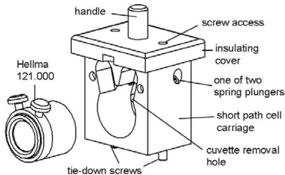
**Figure 2. Short-path cuvette carriage and Hellma 121.000 cuvette**
