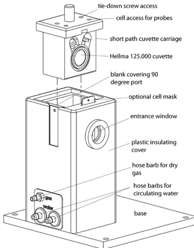
**Figure 3. Placing the short-path cuvette into the CD 250**
