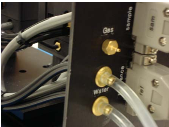
Figure 4. A front panel for the t2x2 Sport showing external connectors for the two water lines and one (optional) gas line, and the two DB15 15-pin cables (labeled “ref” and “sam”). Not all front panels look like this one, and not all t2x2 Sport versions include a front panel.
