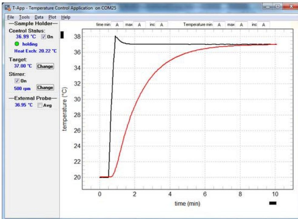
The image above shows the T-App Application window as it would appear using a **TC 1 Temperature Controller** with a Series 400 thermistor probe attached (with the thermistor tip in the stirred sample).
