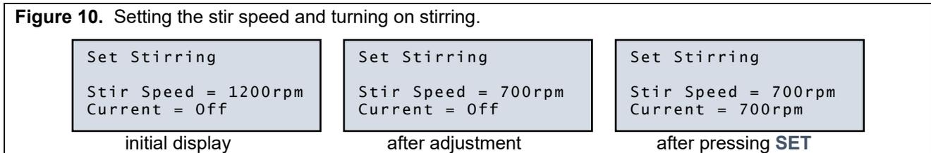
Press the **right arrow** twice to go to the **STIRRING** display, which will look like the "initial display" in **Figure 10**. Then use the **up arrow** and **down arrow** buttons to adjust the "Stir Speed" parameter to 700 rpm. The display will be equivalent to the "after adjustment" example in the figure. Then press **SET** to turn stirring on (and return to the **MAIN** page with "Stir On" at the bottom). The "after pressing **SET**" in **Figure 10** shows what
