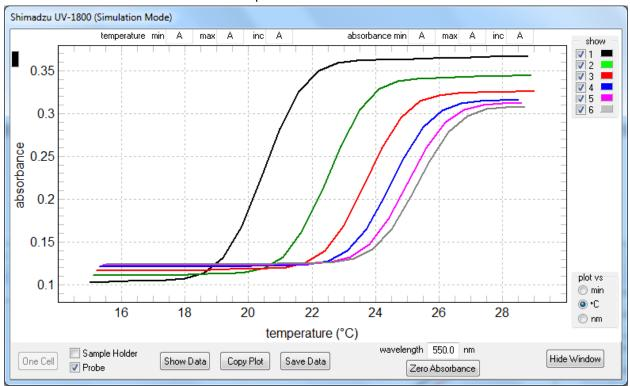
The three radio buttons in the lower right corner of the plot can be used to change the horizontal axis variable to time (min), temperature (°C) or wavelength (nm). This change can be made at any time.
