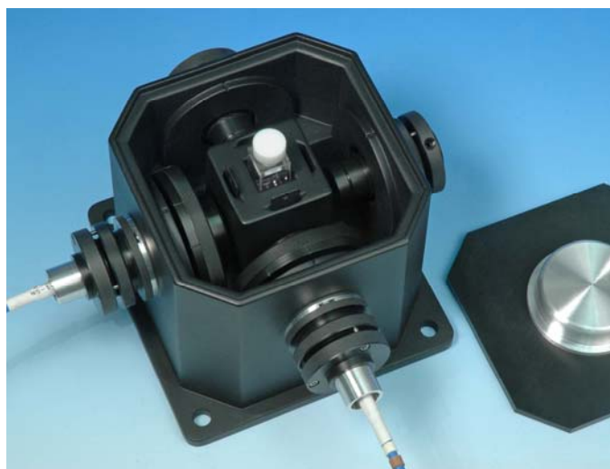
Figure 1 - qpod set up for polarized fluorescence measurements
